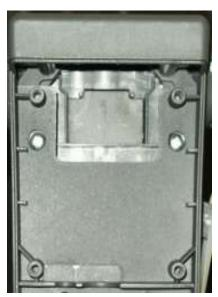
Step 3: Re-install the switch cover assembly. The switch mounting plate will rest on the support plate. Secure all screws and test.
