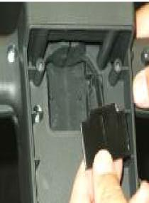
Step 2: Using the molded pins to locate the support plate, install it by pressing it flat against the back of the housing. It will hold itself in place.
